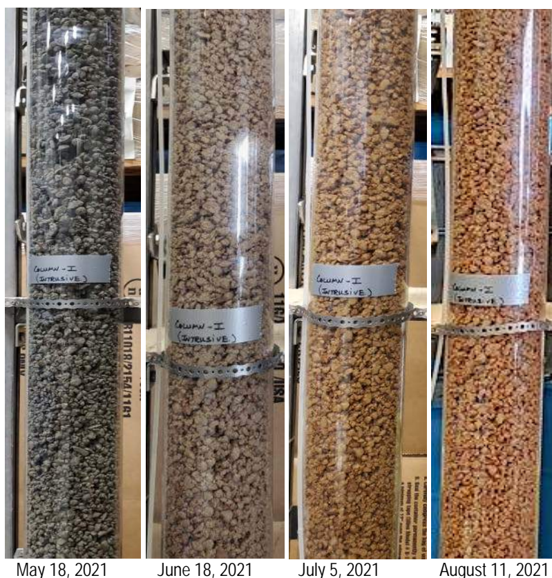
Figure 1-2: Column of Intrusive Composite Sample Under Oxidation
