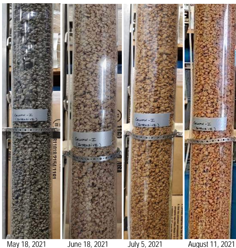
Figure 13-2: Column of Intrusive Composite Sample Under Oxidation
