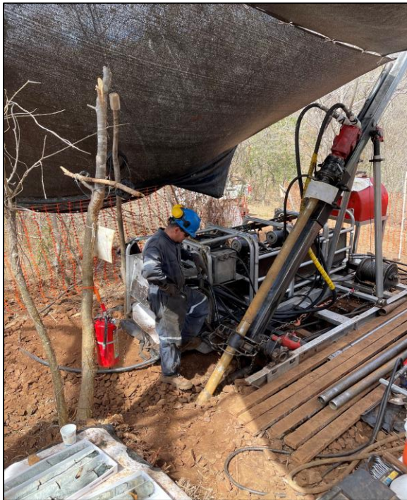
Portable rig for minor environmental impact
